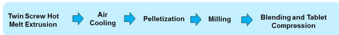
Figure 1: Process Flow for ITR-ASD Tableting
