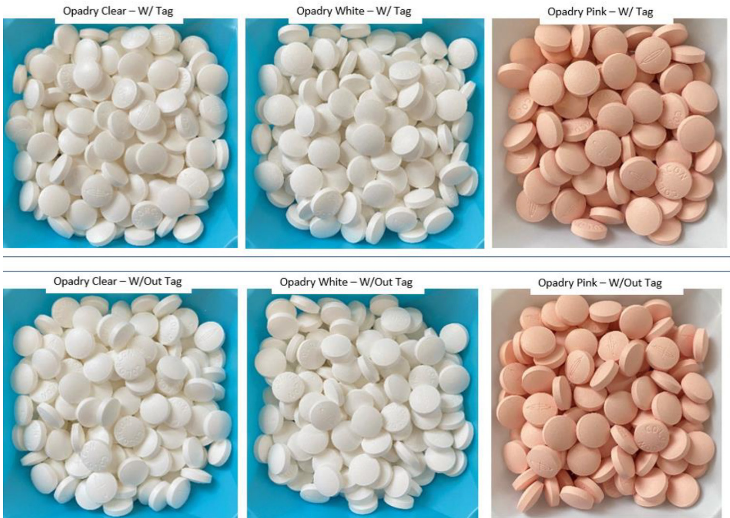
Figure 1. Opadry Coated Placebo Tablets, With and Without Silica-Based Microtaggants
