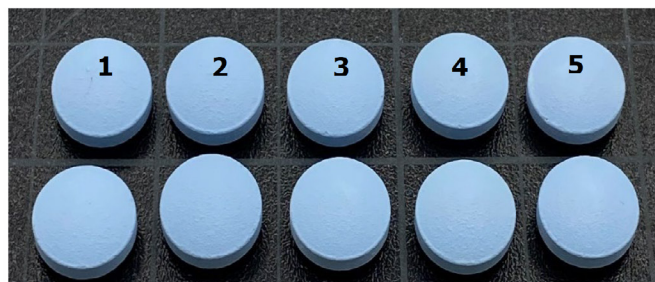
Figure 6. 4% Top-coat Weight Gain Tablets After Washing Method: T=22 Hours in Light Chamber.
