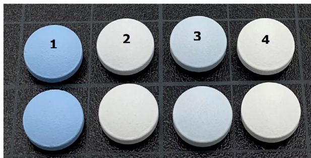
Figure 3. Tablets with 4% Weight Gain Top-coat
