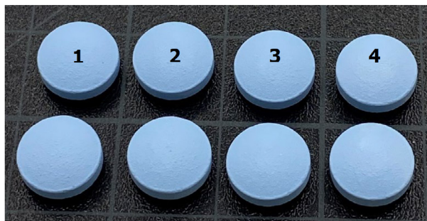
Figure 4. Tablets with 4% Weight Gain of Top-coat, Before and After Washing Method: T=0
