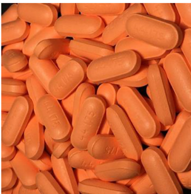
Figure 4: APAP Caplets Coated in the 24" Pan with Pigmented Opadry EZ at 18% Solids
