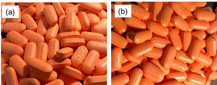
Figure 5: Image of Placebo Caplets Coated on the 48" Pan with (a) Pigmented Opadry EZ followed by (b) Clear Opadry EZ
