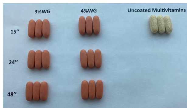
Figure 4: High Productivity/ High Opacity TiO 2 Free Film Coating at 3% and 4% WG using 27.5% Solids
