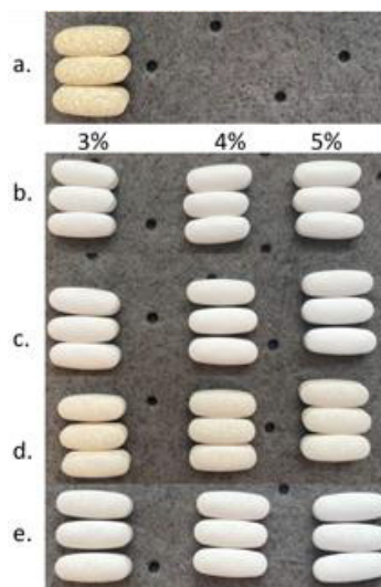
Figure 1. (a) Uncoated Multivitamin, (b) Multivitamin Tablets coated with Nutrafinish TiO 2 , (c) Nutrafinish High Opacity, (d) Experimental, and (e) Nutrafinish Label Friendly
